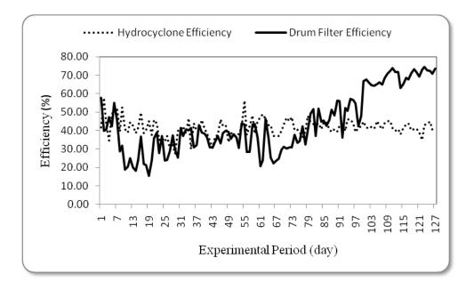
Fig. (6) The efficiency of the removal settleable and suspended solids (%)
