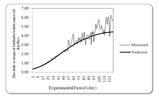
Fig. (3) The daily average of settleable solids removed by hydrocyclone (kg/day)
